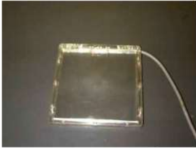
An exposure-area product detector used in radiography.
