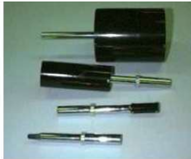
A range of ionisation chambers of different volumes using for measuring radiation exposure.
